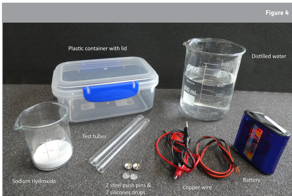
↑ Equipment needed for building an electrolyser
